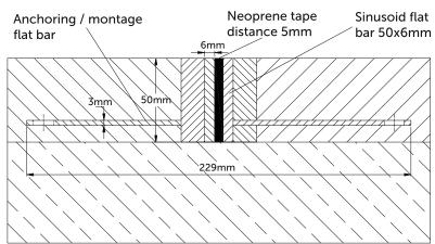
Conecto Sinus are reparation joints designed for cracking floors. Sinusoid construction provides two-level movement which prevent deeper cracking of the floors. Properly installed Conecto Sinus joints eliminate resultant damages and prevent in case of further damages. Properly secured with Conecto Sinus joints floor will not cause vehicles damages and ward off deep cracks which could prevent further usage of floor. Standard length = 2.4 meters.
